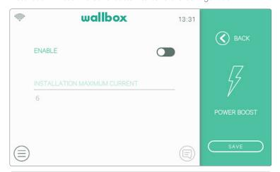
Check the Notification area by pressing the Notification button on the Dashboard to view the status of the Power Boost.
