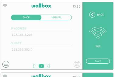
The network parameters are obtained automatically from the network's DHCP server and can be entered manually.
